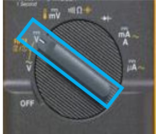
4. Use the DC voltage setting. The polarity of the probes doesn't matter too much, it will just read a negative voltage if reversed. Meters may vary, but look for the V with a straight line over a dashed straight line.
