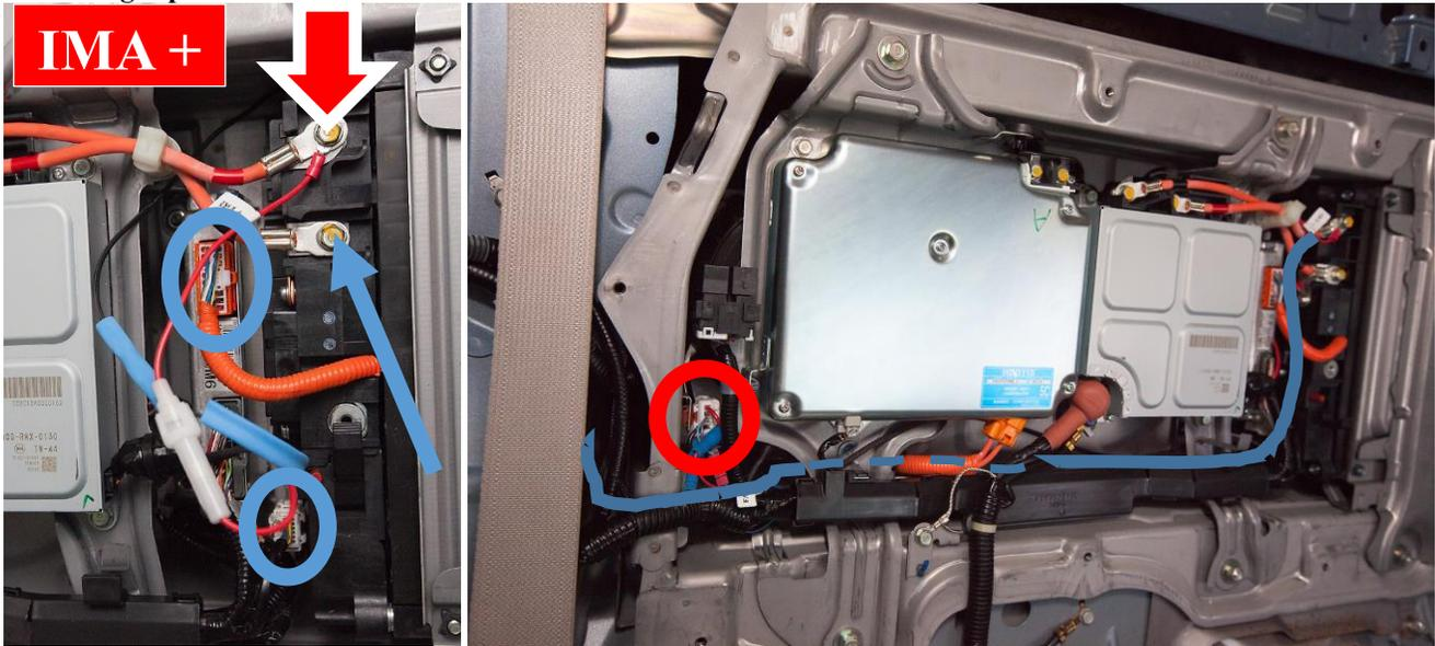
17. Remove the IMA cooling fan connector (red circle), **right picture above**.
