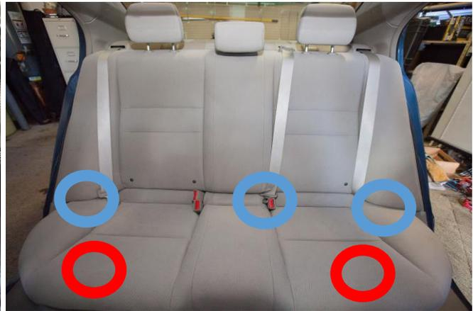
3. Remove the IMA switch cover plate, two T30 bolts (blue circles), left picture below.
